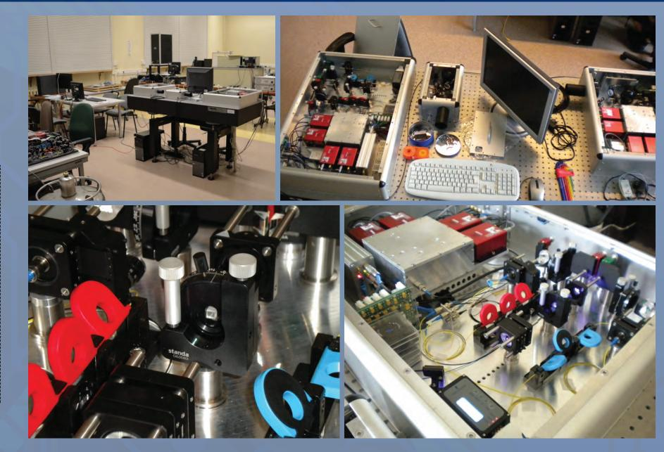
The entangled pairs of photons are provided by parametric down conversion II (PDC) in BBO crystal - EPR S405 Quelle (Austrian Institute of Technology - AIT). Mutually orthogonal, V and H polarized states of photons are entangled on intersection of two cones of transmission of PDC pair produced in birefringent BBO crystal.
