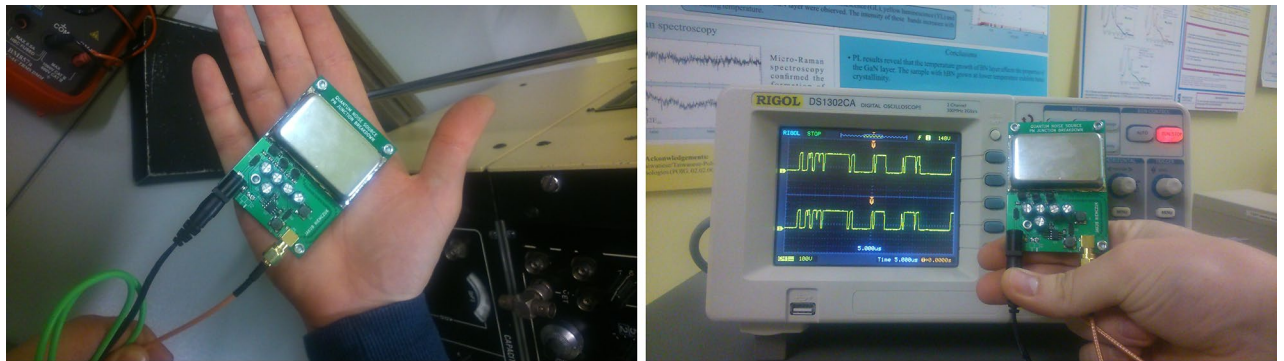
Figure 3. JUR01 quantum random number generator after removing the cover. Generator performance 4Mb/s of random binary code (on the right panel visible signal 0,1 on the oscilloscope screen).
